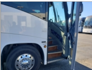
ENTRY WAY STEPS AT FRONT DOOR
